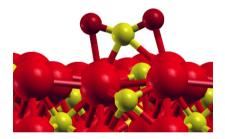
Structure of adsorbed CO<sub>2</sub> on a representative iron carbide surface from preliminary DFT results
