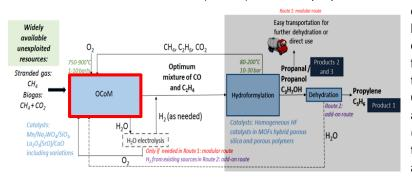
of striving for low  $CO_x$  formation or high  $C_2$  yield, OCoM seeks to obtain a  $CO/C_2H_4$  mixture for further application. As shown in the figure, OCoM involves high  $CO_2$  containing gas (e.g. bio-gas) as feedstock and byproduct (mainly  $CO_2$ ) recycling. Owing to the abundance of  $CO_2$  in OCoM and for the purpose of achieving for OCoM
