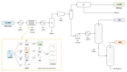
favorable selectivity profiles (i.e., BD + high-value and easy-to-remove side product(s)) were obtained [2]. To evaluate its industrial potential, a preliminary 200 kt/a process flowsheet (see figure) and a detailed kinetic model are currently being developed in our group.
