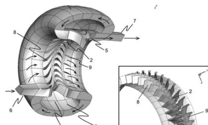
Figure 1: Electrified rotor stator reactor.
