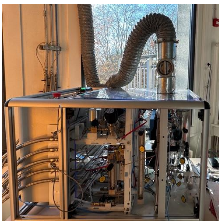
Figure 1. Portable reactor for the catalytic tests.
