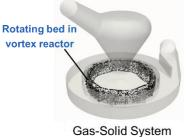
adsorption-desorption cycle of various sorbents under novel regeneration methods within a vortex reactor system, paving the way for optimized and cost-effective DAC technology.
