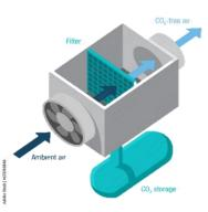
technology can be optimized in the areas of air contactors, solvents/sorbents and regeneration methods<sup>1</sup>. This need for process intensification (PI) of direct air capture led to the conception of this project which is based on the vortex technology.
